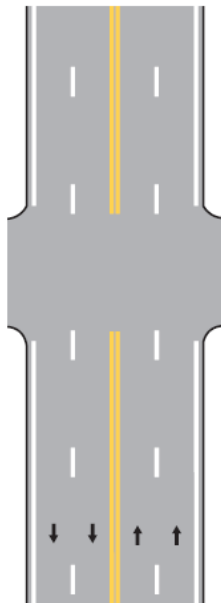
A - Typical multi-lane, two-way marking
